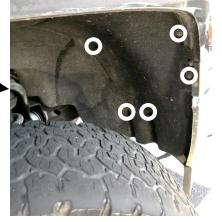
(bolts not in frame). Remove the single bolt at the other end of the support and place the bar aside. Remove the six bolts shown by the white arrows. (dashed white circle shows bolt location behind support bar)
